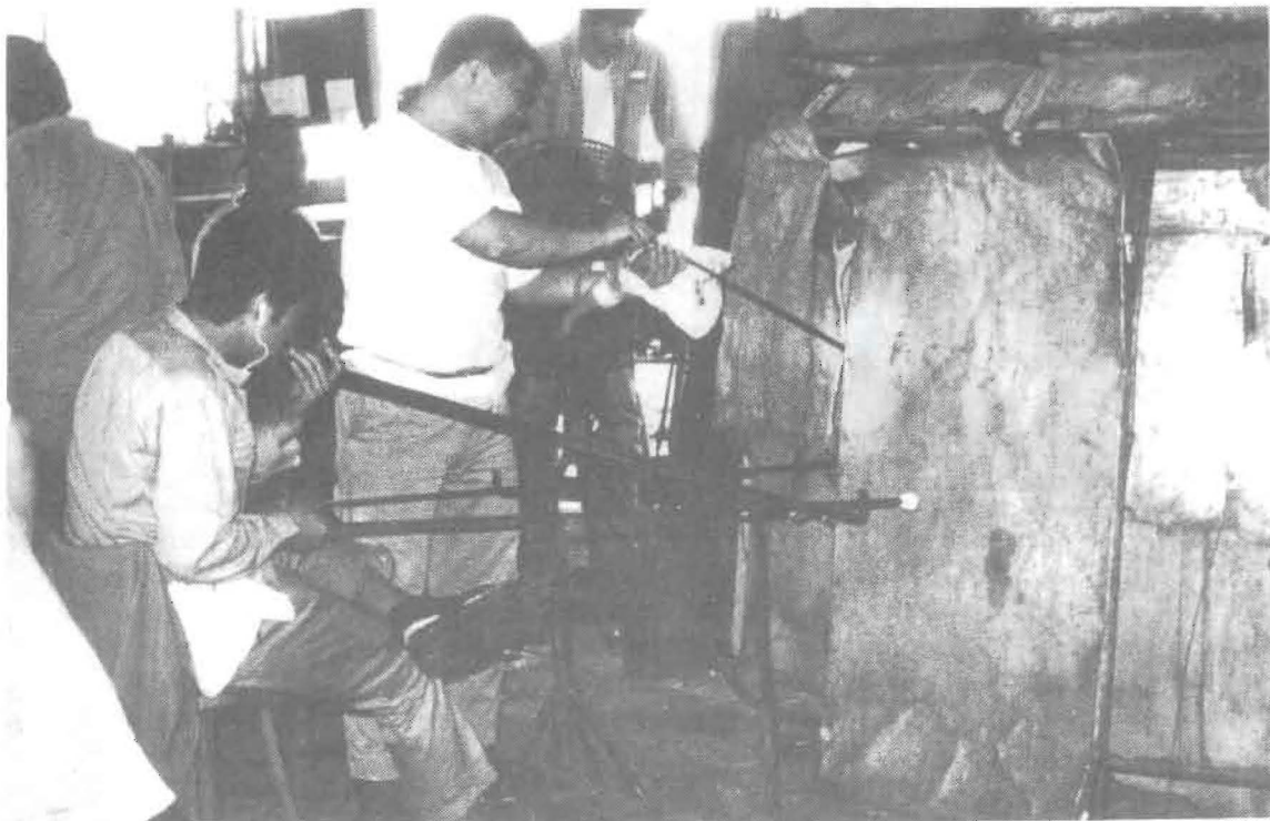
Blowing first bubbles in multiple - two pipes in the mouth and three others cooling.
