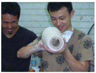
The 1<sup>st</sup> day & a half was spent designing and creating moulds using the common plaster/silica/water mix and the pre-mixed Japanese product G2/water; it was a great way to compare the two and all its properties. We also used two different glasses (soda/lime) in cullet & frit form – 1 from Germany, 1 from Japan, the clarity of Japanese glass was far superior, however some of the class found that it had a cold appearance.
